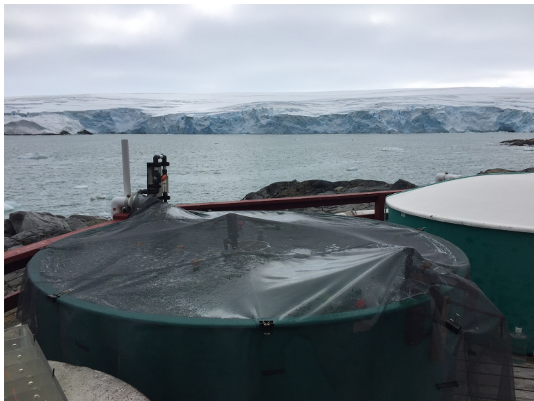
Figure 7.2. Image of the glacial meltwater microcosm experiment incubation aquarium located on the Palmer Station deck. The Marr Glacier can be seen in the background.
